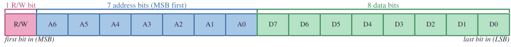
Figure 2. Serial register interface. (a) The sixteen single-byte registers that configure the neuron, grouped by function: control and refractory, feedback polynomial, seed, threshold, decay, status, and the eight activation-table entries. (b) The sixteen-bit serial frame, with one read-or-write bit, seven address bits sent most significant first, and eight data bits.
